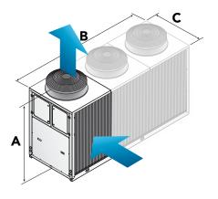
EVR - Outdoor unit with double heat exchanger and vertical airflow
