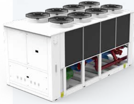
AIR COOLED CHILLERS FOR OUTDOOR INSTALLATION equipped with inverter screw compressors, axial fans and microchannel condensing coils RAH MC VS Serie Cooling capacity from 306 kW to 1555 kW
