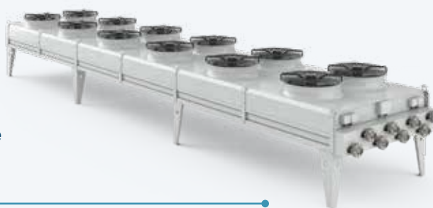
FLAT DRY COOLER Flat dry coolers with axial fans for outdoor use Cooling capacity from 7 kW to 630 kW
